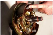
6) Install the brakes shoes and secure them with the springs. Remember to reconnect the Bowden brake cable.
