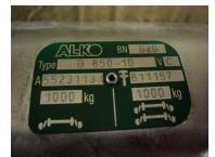
The **brake type** is stamped on the brake backing plate (aft side of the
