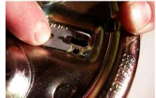
4) ... and pushing the retainer clip on the aft side of the backing plate. Disconnect the Bowden brake cable new springs! and remove the old brake shoes.
